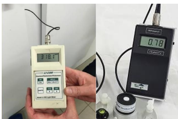
Figure 4: a) Li250A light meter measuring the PPFD in a growth chamber. Photo: Martin Knoop b) Red/Far-Red sensor from Skye (UK). Photo: www.skyeinstruments.com
