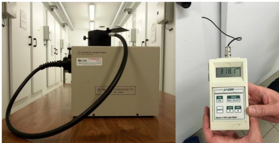
Figure 8: Optronic model 756 spectroradiometer for spectral measurement composition (left) & Quantum meter used to measure the light intensity (right) (Knoop, 2019)
