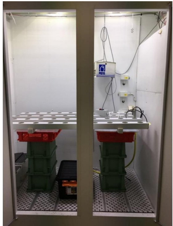
Figure 6: Chamber setup with an NFT Hydroponic System (Knoop, 2019)
