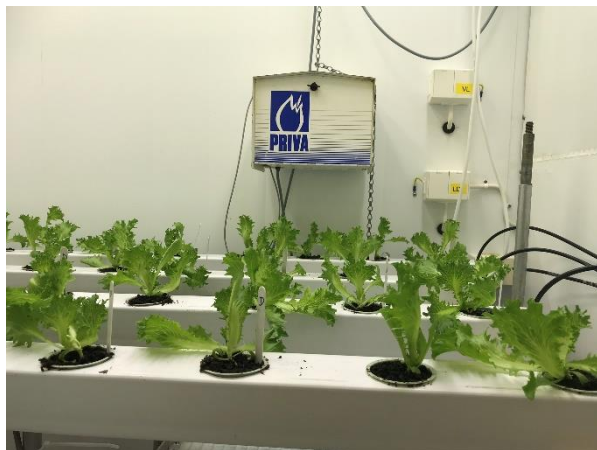
Figure 7: Priva aspirated sensor box along with the planted lettuce in gutters. Photo: Niveditha Umesh Katyayini
